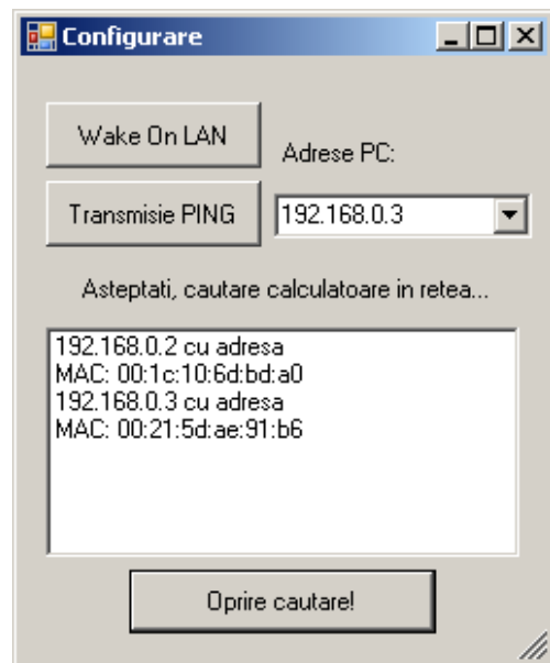
Fig 5. Network discovery stage using SendARP
